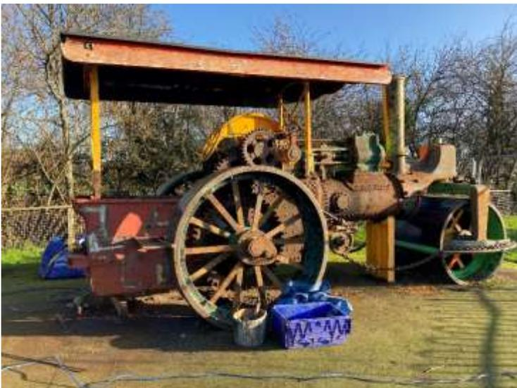
*Works can be seen to rear of engine where new steel has been installed.*
