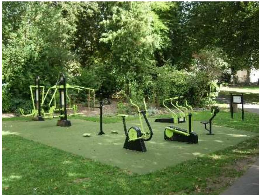
The gym site comprises the following equipment placed within a Notts Sward safety surfaced area. Whilst critical fall heights are very low (less than 800 mm) the safety surface helps to prevent erosion of the former grass surface and does provide some softening of any accidental fall. It is comprised of the following equipment: -
